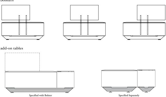
Add-on tables can be specified as part of the bench, or be ordered separately as required. When the table is ordered with the bench it has one continuous base, when it is ordered separately, the bench and table will have two separate bases.
