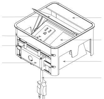
Top Plate and Data/Electrical Box are finished in clear Anodized Aluminum
