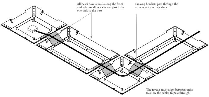
When planning with electrical, Teknion dna units must be linked together. Reveals alone the fronts and sides alone. Cables to pass from one another to the next and accommodate linking brackets.
