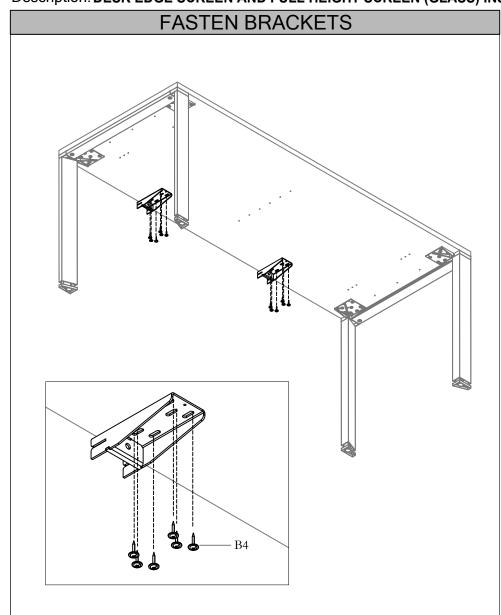
STEP 2: Fasten Bracket Weldments to underside of Worksurface with pan washer screws provided.
