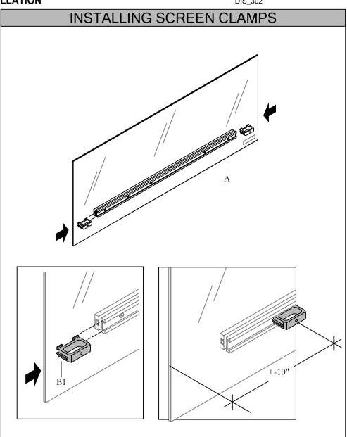
Step 3: At each end of the metal extrusion slide in the two Screen Clamps. Position the Clamps so that they are aligned with the brackets underneath the worksurface.
