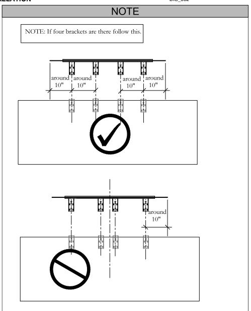
NOTE: Brackets should be placed +/- 10" in from the edge of the **GLASS**. If there is storage under the worksurface, adjust the location of the bracket as long as it does't pass the midpoint of the Glass.
