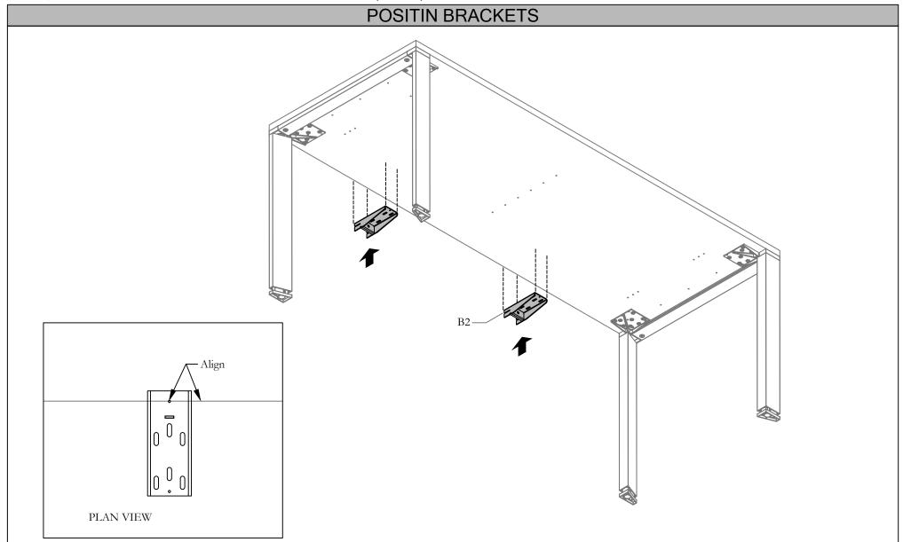
STEP 1: Position Bracket so the hole on the top surface of the Bracket is aligned with the edge of the Worksurface (see above). IMPORTANT! The Brackets must be PERPENDICULAR to the Worksurface edge.
