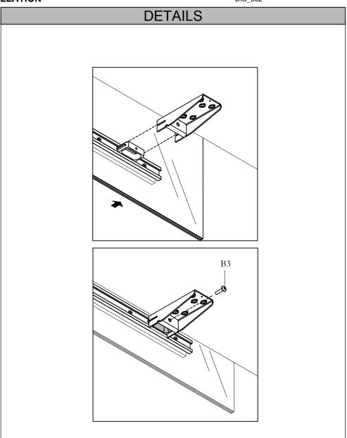
STEP 4: To install Screen on edge of worksurface insert Screen Clamps inside Weldment Brackets. One person should hold Screen, while another fastens Brackets and Clamps together.
