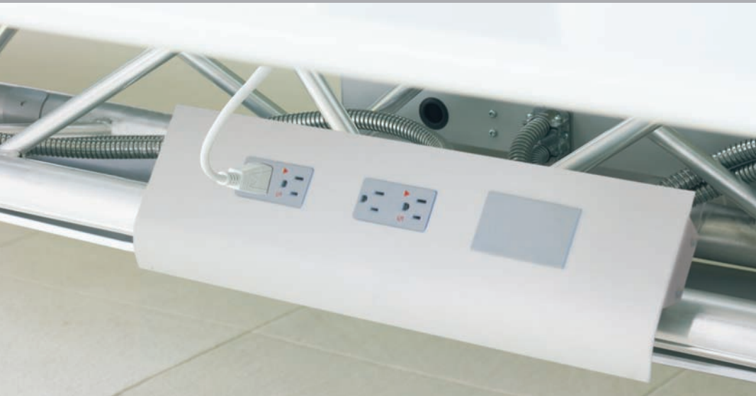
^ POWER/COMMUNICATIONS BOX TRUSS-MOUNTED Mounts to the truss and provides below-surface plug-in to power and data with standard or high-capacity options.
