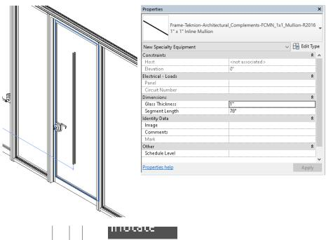
3. Corner Mullions are also placed as Work plane based specialty equipment. Ensure that the Mullion Family is aligned to each side of the glass correctly after placement
