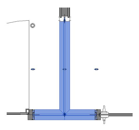
Although these are stand-alone elements and are not part of the curtain wall system family, they share parameters allowing for seamless customization. i.e. "Glass Panel Offset" parameter.
