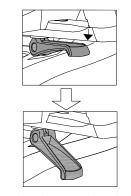
To adjust the arm width push the lever down and slide the arm to the desired position. Push the lever up to lock the arm in place.
