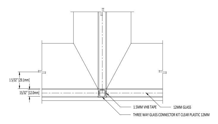
OFFSET GLASS THREE WAY CORNER CONNECTION WITH CENTERED GLASS - 12MM PLASTIC
