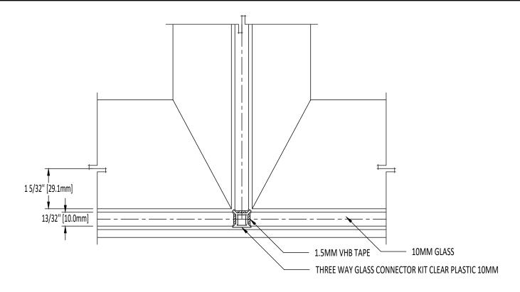
OFFSET GLASS THREE WAY CORNER CONNECTION WITH CENTERED GLASS - 10MM PLASTIC
