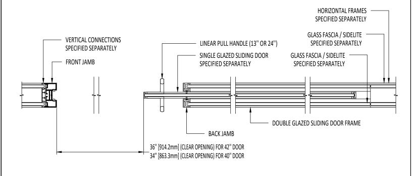
HORIZONTAL SECTION THROUGH OPEN SLIDING DOOR - DOUBLE GLAZED FRAMED - SPLICE POINT
