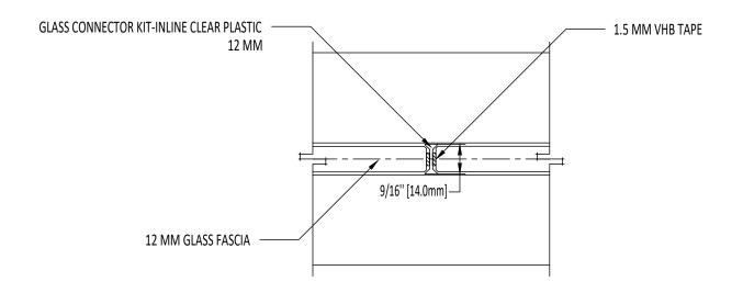
GLASS CONNECTOR KIT-INLINE TAPE - 12 MM
