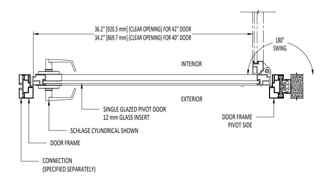
HORIZONTAL SECTION THROUGH SINGLE GLAZED PIVOT DOOR
