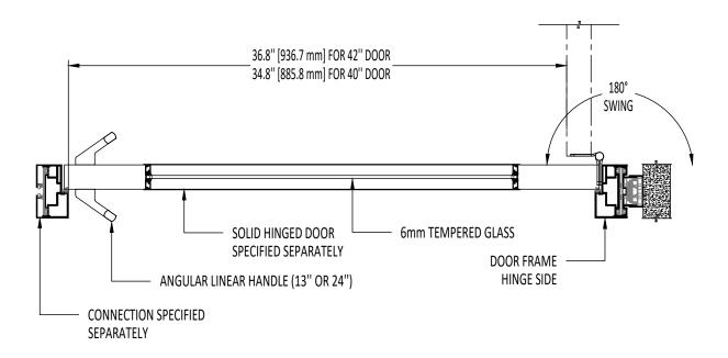
HORIZONTAL SECTION THROUGH SOLID HINGED DOOR WITH GLASS INSERT
