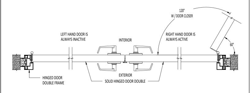
HORIZONTAL SECTION THROUGH SOLID HINGED DOOR - DOUBLE
