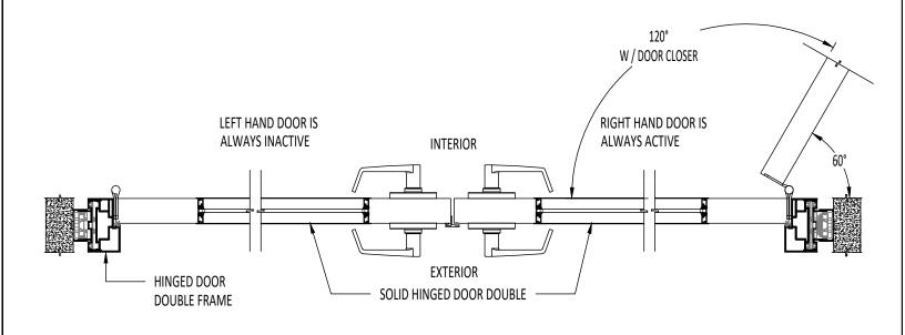
HORIZONTAL SECTION THROUGH SOLID HINGED DOOR WITH GLASS INSERT - DOUBLE
