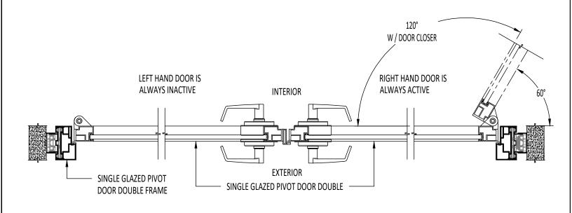
HORIZONTAL SECTION THROUGH SINGLE GLAZED PIVOT DOOR - DOUBLE OPEN
