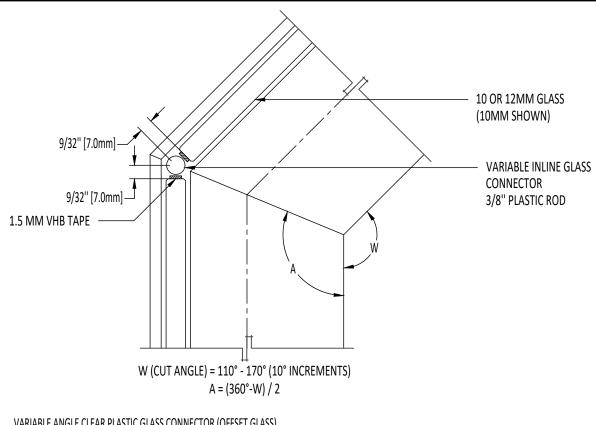
VARIABLE ANGLE CLEAR PLASTIC GLASS CONNECTOR (OFFSET GLASS)
