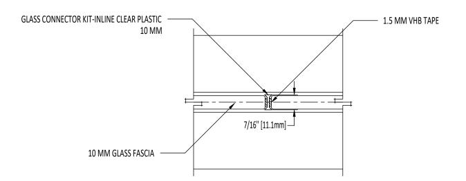
GLASS CONNECTOR KIT-INLINE TAPE - 10 MM
