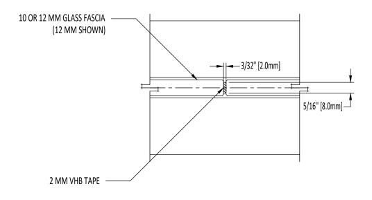
GLASS CONNECTOR KIT-INLINE TAPE - 12 MM
