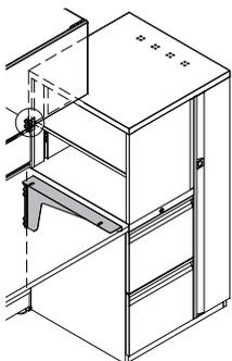
**Supporting Locker Bracket (LLB)** used in combination with Ledger Storage Lockers (LSLF, LSLS) 24" wide only provides a support at the end of a run of panel-mounted worksurfaces
